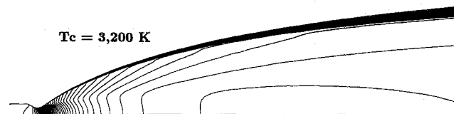
Fig. 7 Static temperature contours of the reference nozzle ( T_c = 3200 K).
